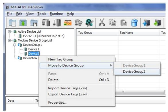
2. The Modbus device will be moved to the target device group.
