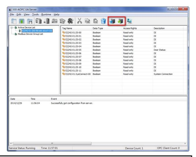
NOTE The first time you use MX-AOPC UA Server, we recommend turning off the Windows Firewall and then checking to see if MX-AOPC UA Server is able to receive active tags. If it can, turn the Windows Firewall back on and check it again. If MX-AOPC UA Server does not receive any active tags after you turn on the Windows Firewall, add aopcservice.exe in the Firewall Inbound Rules, and set it to Allow for Private, Public, and Domain network profiles.
