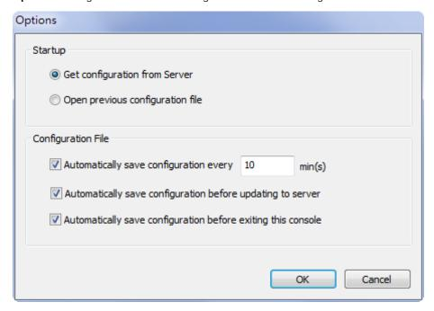
**NOTE** If **Automatically save configuration every xx min(s)** is enabled, the configuration file will be automatically saved only when a file name is defined. Be sure to save your configuration file after creating a new project file.
