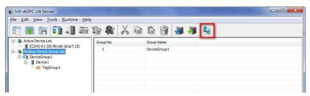
The device tree in the left panel should be the same as the tree displayed by the configuration console. Click a tag group name to display the group's tag values in the right panel.
