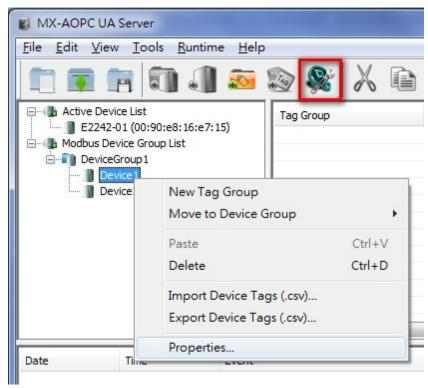
**NOTE** You are not allowed to cut, copy, or paste a Modbus device.
