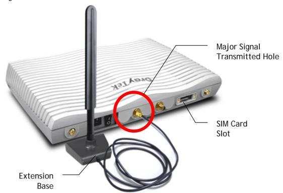
Note, if only one antenna shall be installed, please use the mounting hole (major signal transmitted hole) near to the power switch.
