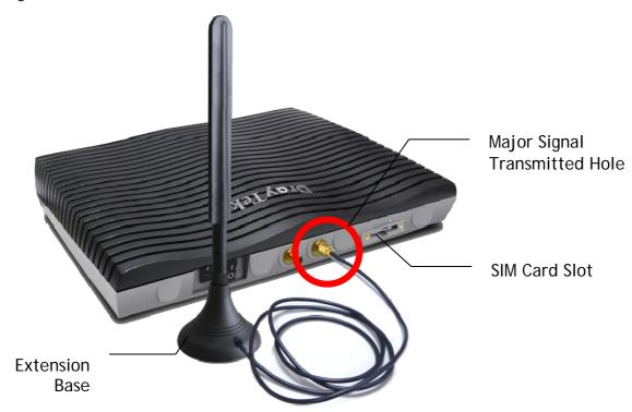
Note, if only one antenna shall be installed, please use the mounting hole (major signal transmitted hole) near to the SIM card slot.
