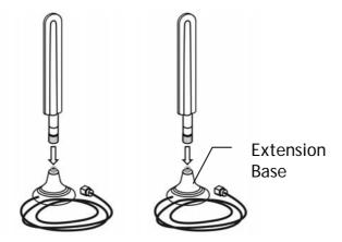
There are two mounting holes for installing antennas with extension base on Vigor router. Please install them as shown below.
