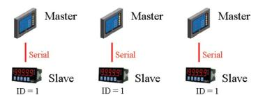
The MGate MB3000 can connect to each serial slave, so Ethernet SCADA masters will be able to control them. However, since slave IDs cannot be repeated in a system, we will need to change the IDs of some of the slaves in order to integrate them into a single network, as follows:
