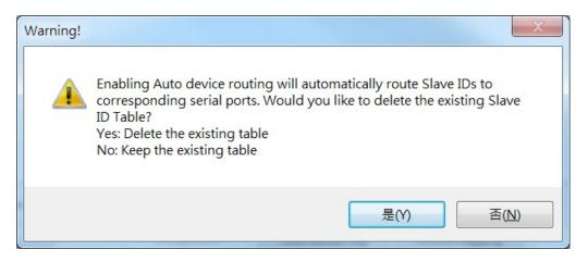
Click **Yes** to delete the existing (factory default or user-set) routing table; the auto routing mechanism will automatically find the correct serial port that connects the target Modbus device. Moreover, if a device is added to the gateway later, the gateway can also route it correctly. Note that the routing table will be clear as illustrated below.
