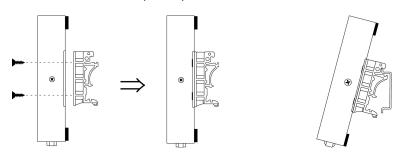
**Mounting on the wall:** Place two screws in the wall and slide the unit onto the screws as shown. The head of each screw 6.5 mm or less in diameter, and the shaft should be 3 mm or less in diameter. Make sure to leave about 2 mm of space between the head and the wall.
