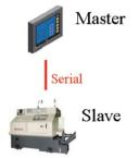
An advanced multiport MGate model (MB3270) can be inserted into the serial system, with the slaves connected to one serial port and the master to another serial port. The advanced gateway allows Ethernet masters to communicate with the serial slaves, and it also provides a serial redirector function that simultaneously allows the serial master to continue controlling the slaves.
