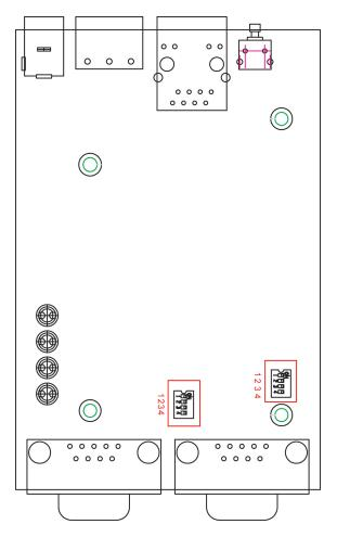
**To add a 120**  $\Omega$  **termination resistor,** set switch 3 on the port's assigned DIP switch to ON; set switch 3 to OFF (the default setting) to disable the termination resistor.
