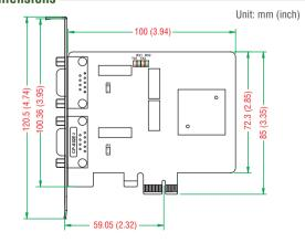
602E-I CAN interface board uses the NXP SJA1000 and transceiver PCA82C251, which provide the bus arbitration and error detection. The -40 to 85°C wide operating temperature (CP-602E-I-T only) and 2 kV isolation make the boards suitable for use in harsh industrial environments.
