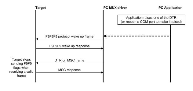
Note: If the valid frame is a DATA frame, the embedded module does not detect any DTR change and sleeps on again with the PSC frame.
