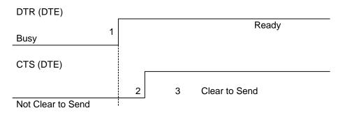
**1:** The application raises its DTR signal to indicate a ready state (meaning DTE wants to communicate with the DCE).
