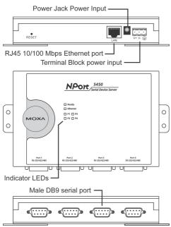
Reset Button—<u>Press the Reset button continuously for 5 sec to load</u> <u>factory defaults:</u> Use a pointed object, such as a straightened paper clip or toothpick, to press the reset button. This will cause the Ready LED to blink on and off. The factory defaults will be loaded once the Ready LED stops blinking (after about 5 seconds). At this point, you should release the reset button.
