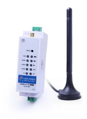
USR-DR502 is a LTE Cat 1 communication modem, which supports LTE and GSM. USR-DR502-E covers the mainstream frequency bands of European operators. It has perfect software function, supports TCP/UDP transparent transmission, SIM transmission, HTTPD Client mode and AT command configuration. In addition, it is simple to configure has high reliability and built-in hardware watchdog, supports FOTA upgrading.
