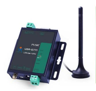
USR-G771 is an LTE CAT 1 cellular modem, which supports LTE and GSM. USR-G771-E covers the mainstream frequency bands of European operators. It has perfect software function, supports TCP/UDP transparent transmission, SMS transmission, HTTPD Client mode, and AT command configuration. Also, it is simple to configure, has high reliability and built-in hardware watchdog, supports FOTA upgrading.
